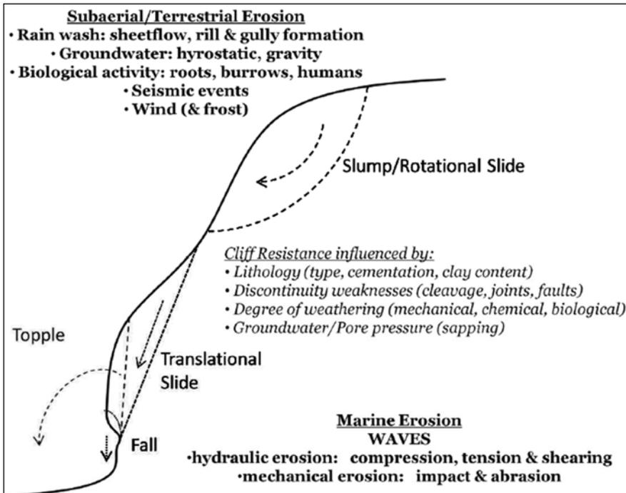
Figure 1. Illustration of typical failure modes in coastal cliffs, the subaerial and marine forces that drive them and the inherent properties of the cliff material which contribute to resisting erosion.
