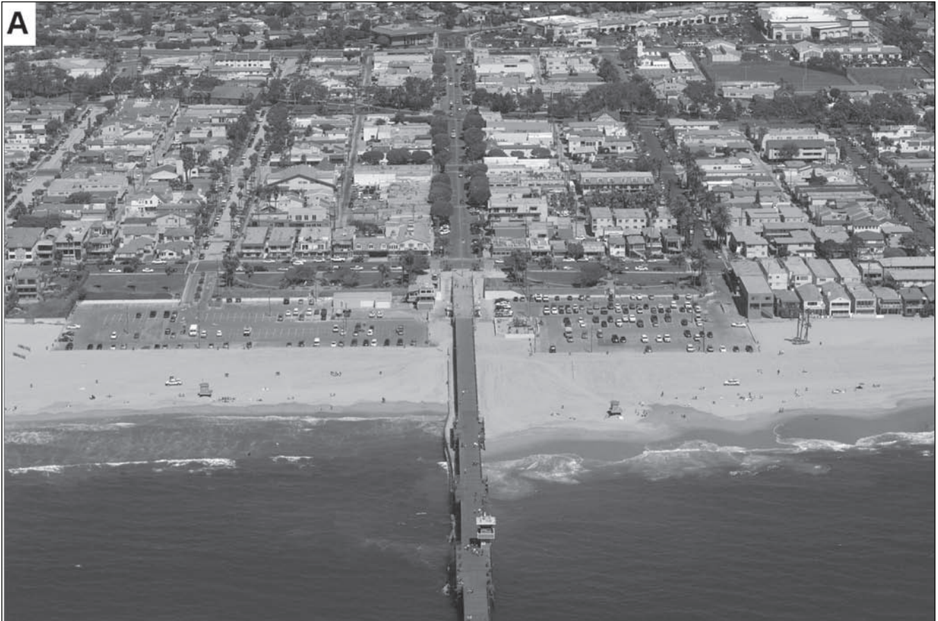
Figure 5. (A) Oblique aerial image of Seal Beach in Orange County, California (Adelman and Adelman 2009). (B) Seal Beach today, shown with the 1932 shoreline position prior to artificial nourishment and the later construction of the groin under the pier in 1959 (Wiegel 1994). This area is characterized by net littoral drift to the north (Patsch and Griggs 2007). The site was regularly nourished with \sim 250,000 yd 3 of sand every 1-2 years from 1950-1970, and again several times in the 1980s (Coyne 2000). This is an example of how existing structures such as wharves and piers could be modified to play a larger role in future nourishment efforts.
