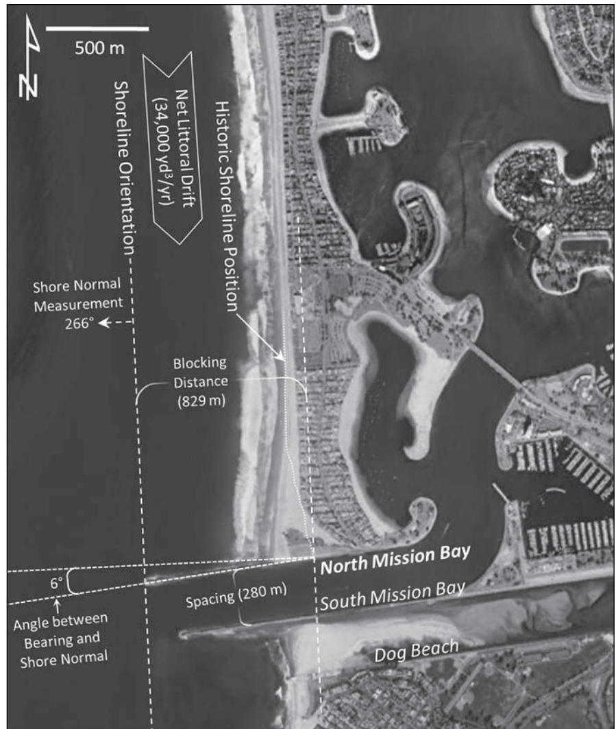
Figure 2. Image depicting the measurements used in the statistical analysis of structures, shown for the North Mission Bay Jetty. The inland extent of the structure is defined as the position where the historic shoreline intersects with the structure. The shoreline orientation is measured along the shore normal in compass degrees from true north. The net littoral drift rate is obtained from Patsch and Griggs (2007).
