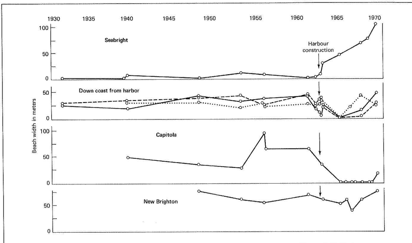
Figure 2. Chronologic changes in the widths of beaches upcoast and downcoast from the Santa Cruz harbor before and after harbor construction.
