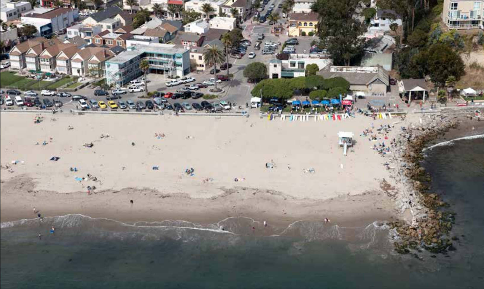
Figure 26. Groin at Capitola along the northern Monterey Bay shoreline that was built in 1969 to restore and stabilize the beach lost when the upcoast Santa Cruz Small Craft Harbor was built. Courtesy: California Coastal Records Project.
