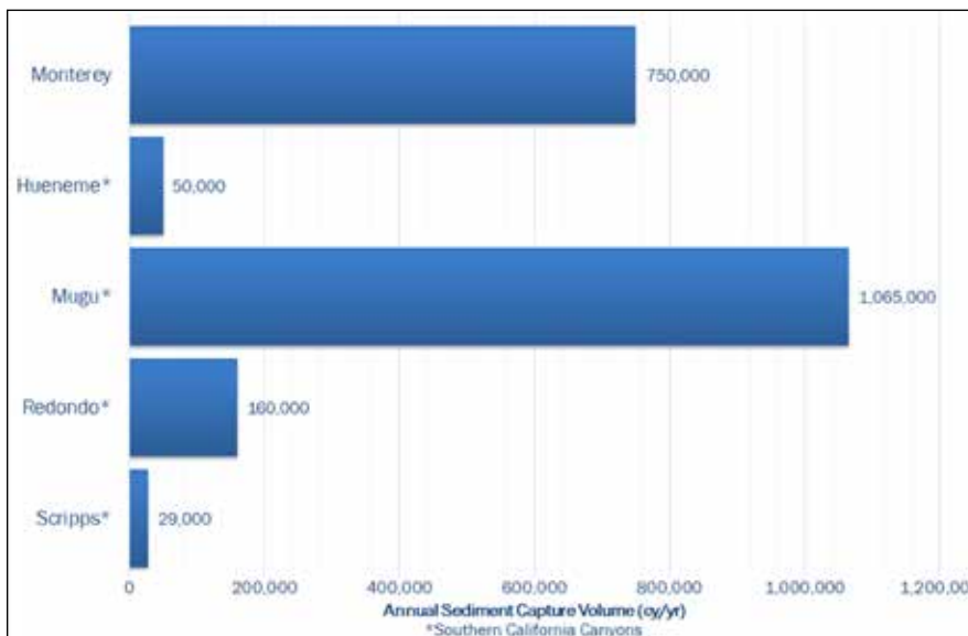
Figure 5 (below). Approximate annual sand capture for submarine canyons funneling more than 10,000 cubic yards of sand per year offshore (Patsch and Griggs 2005; Moffatt & Nichol and Everts Coastal 2009, Everts Coastal 2002; and Everts and Eldon 2005)
