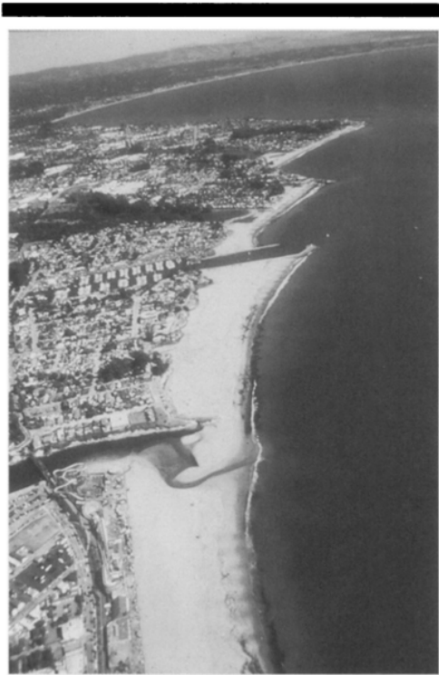
Figure 10. Three headlands and a jetty are responsible for creating the main beaches for the city of Santa Cruz. From top to bottom, Soquel Point, Blacks Point, the jetty of the Santa Cruz small craft harbor, and San Lorenzo Point. Note how the sand trapped by the jetty has extended the upcoast beach further seaward of the natural groin (1997).
