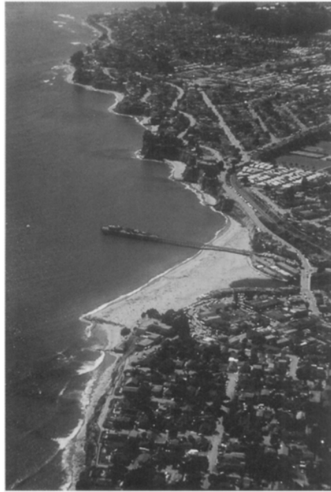
Figure 8. The groin at Capitola has created a nearly permanent year-round beach (1997).
