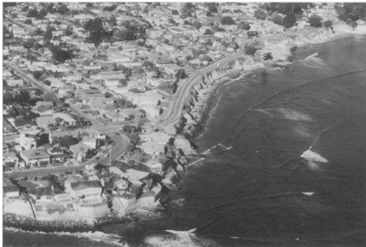
Figure 17. Area of low eroding cliffs between Santa Cruz and Capitola where a seawall is being contemplated. This appears to be an appropriate area for groin emplacement that would form a beach that would both halt bluff erosion and provide recreational area (1989).
