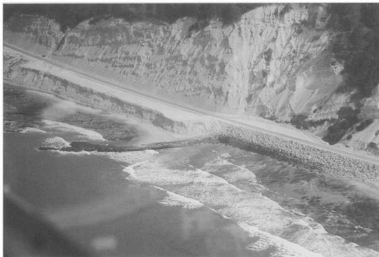
Figure 2. A resistant siltstone bed outcrops in the surf zone and forms a natural groin trapping upcoast sand along the coast between Santa Cruz and Half Moon Bay (1972).
