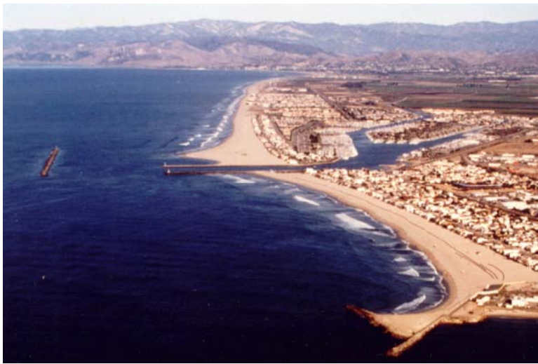
Figure 31. Detached breakwater and salient at Channel Islands Harbor (background); every two years over 2 million cubic meters of sand are artificially bypassed from the salient to Hueneme Beach (out of the picture to the right of the entrance to Port Hueneme in the foreground).
