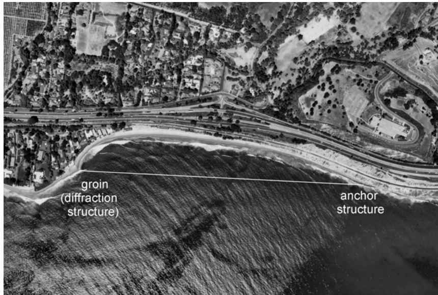
Figure 80. Small hook-shaped bay that formed downcoast of a groin in the natural hooked bay east of Fernald Point.
