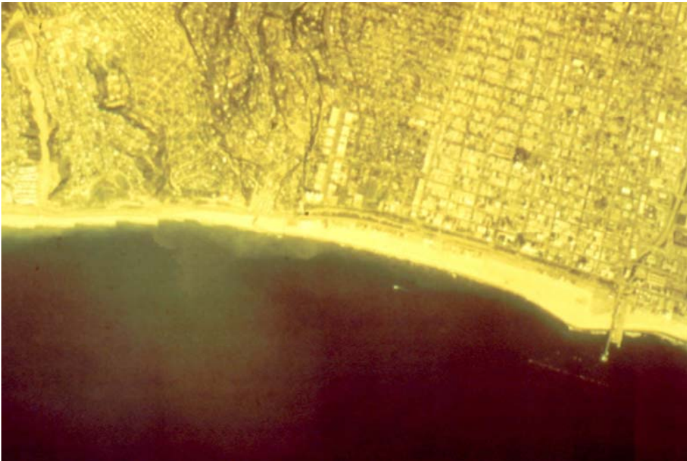
Figure 10. Fillet beach upcoast of the salient that formed in the lee of the Santa Monica breakwater; fillets within the Will Rogers State Beach groins at left (1970's photo).
